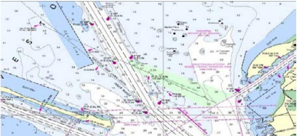
*Note: The Bolivar Roads Inbound Route is 1700 feet wide at its entrance (lower right), 730 feet wide at its exit (upper left) and one nautical mile in length. Range lights assist with staying on the centerline.*
