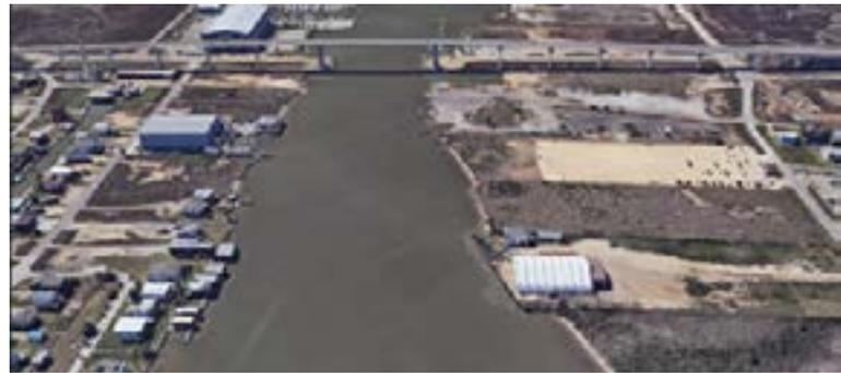
The Surfside Bridge is a fixed bridge located at mile 394 on the Intracoastal Waterway. It has a 73 feet vertical clearance, and a 125 feet horizontal clearance. Mariners must consider the tidal currents, wind, and traffic, when transiting this bridge. When transiting eastbound, make passing arrangements prior to transiting this area because of limited meeting room in the Wiggles. Recreational vessel traffic can be heavy, especially at the bait store just west of the bridge on the north side.
