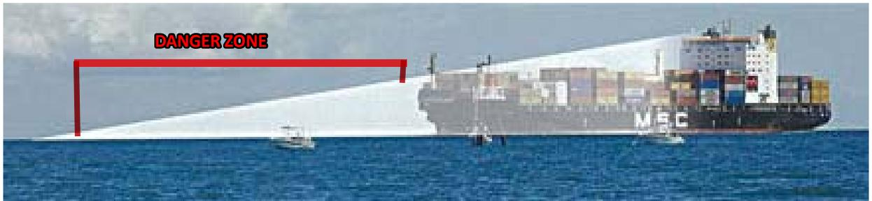
Vessels as large as neo-panamax container vessels (1160'x150') and suezmax tankers (950'x165') regularly transit the HSC. The sheer size of these vessels leads to amplification of hydraulic forces exerted on other vessels in the vicinity, especially tow vessels and barges.
